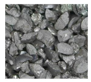
Surface cleanliness is the prime requirement for good holiday-free coating practice. Engineered by combining the best steel with carbon levels high enough to be called iron. Manufactured to precise standards, quick chilled, then heat treated to produce an incredibly hard blasting material. The best abrasive for the toughest jobs. The result is a cleaner surface, with high speed cleaning at a lower cost.
